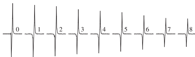
Figure 5. Storage of two-spin order in a spin system. Shown is the high-field doublet of the aromatic protons (ca. 8.5 ppm) of L-tyrosine (4 mM in D_2O ; 16 acquisitions per spectrum). Two-spin order was generated by the pulse sequence of equation (25), subjected to the number of storage cycles ( S_1 + S_2 ) given at the traces, and then read out by a pulse. The spectrum labeled '0' is the control experiment without storage. Further explanation, see text.
