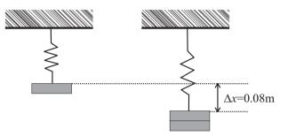
Because the mass is at equilibrium in both cases the net force on the mass is zero, and we can write
